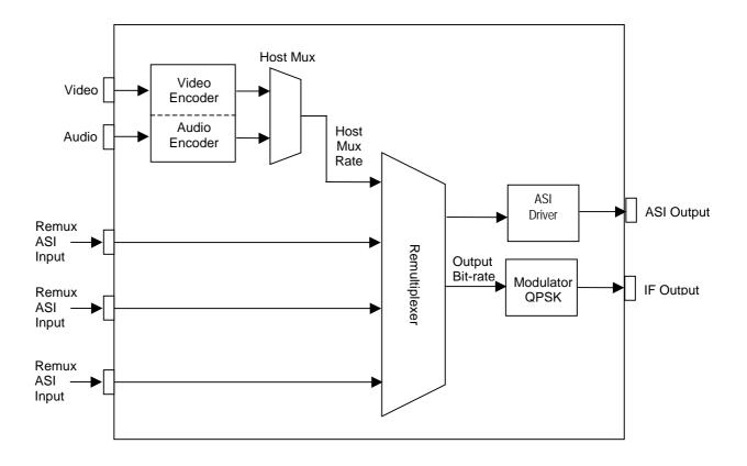
Figure 3.6: Remultiplexer Block Diagram
